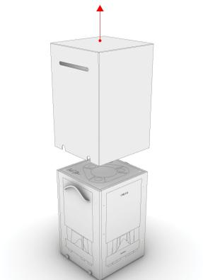
1. Remove cardboard protection box by lifting it upward.
