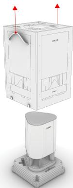
3. Carefully lift and remove the cover from the speaker/case.
